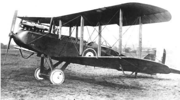
DE HAVILLAND 9 Fitted with one 230h.p. Siddeley Puma engine
