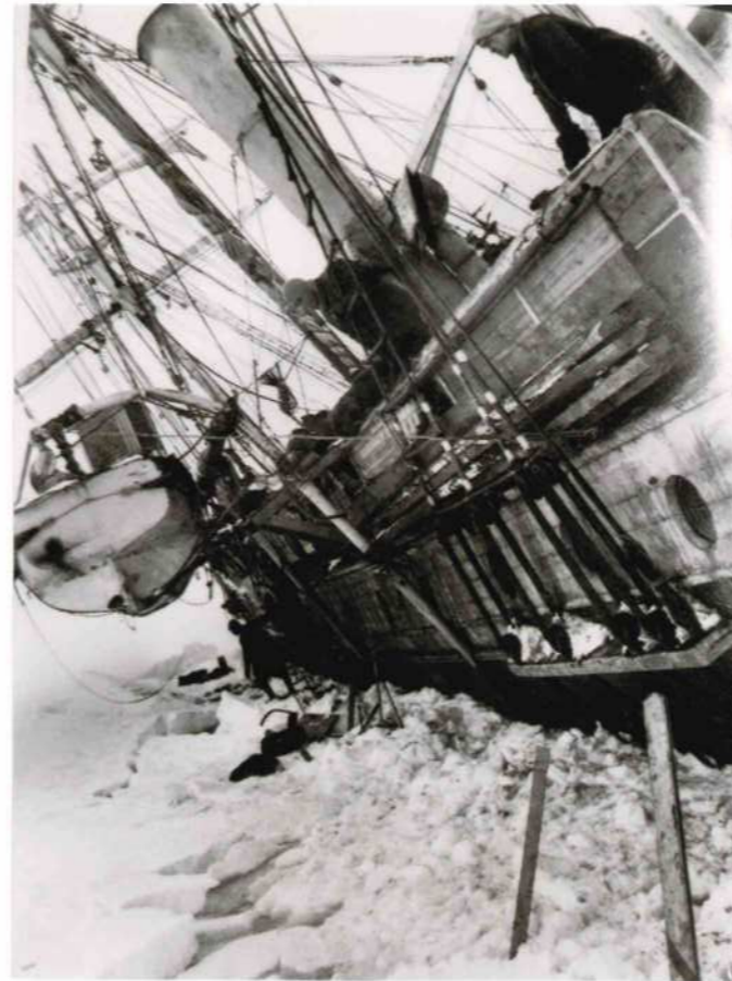
The Endurance keels over as a result of a pressure wave in the sea below the ice.
