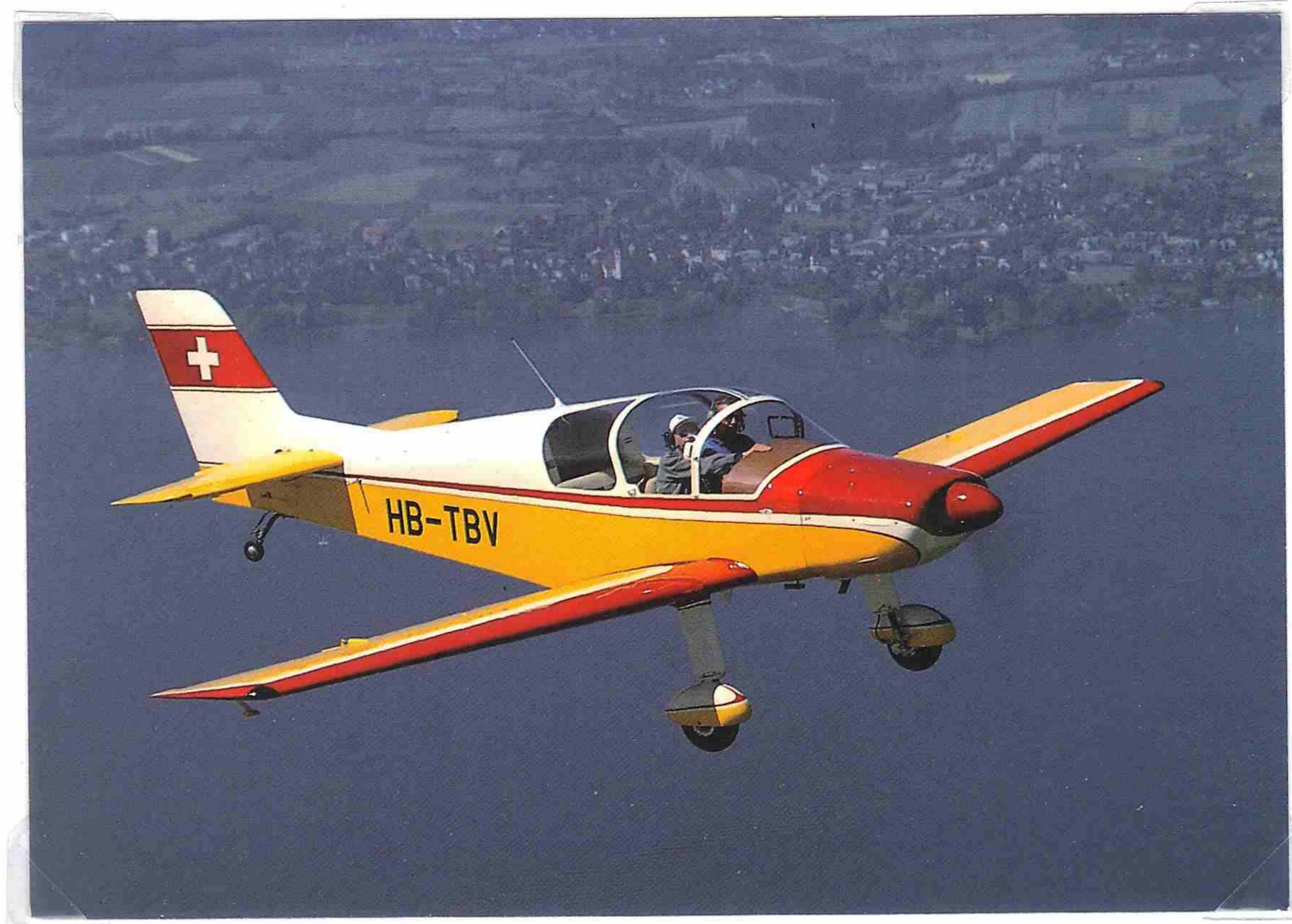
The Pelican U3M is a Swiss four-seat, single-engine aircraft with an extended transparent cabin for good visibility. It has a fixed undercarriage and is a low-wing version. The prototype flew for the first time on May 21, 1963. (Edit: Antique Airplane association, photo: Erich Gandet)
